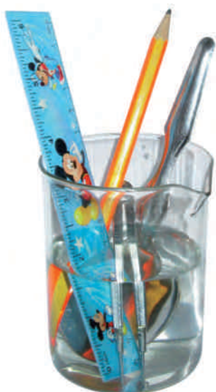
Fig. 3.8 Conduction of heat by different materials
