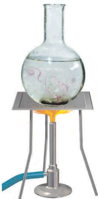
Fig. 3.9 Convection of heat in water
